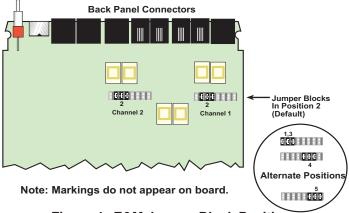
Figure 4. E&M Jumper Block Positions
